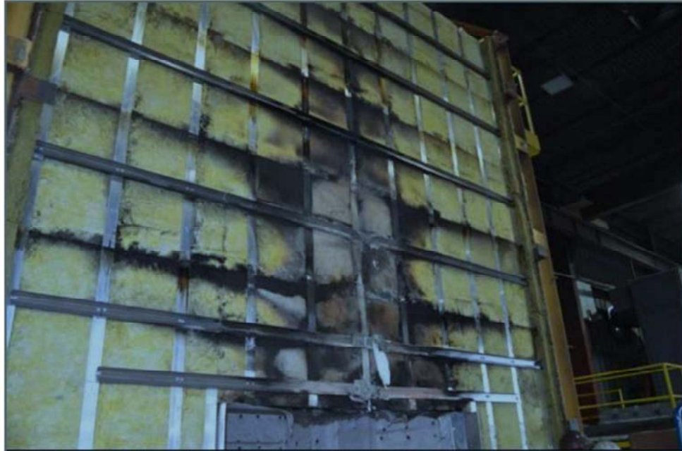
Figure C-16. Post Test Assembly Dissection – Exterior Surface of Mineral Wool Layer after Exposure.
