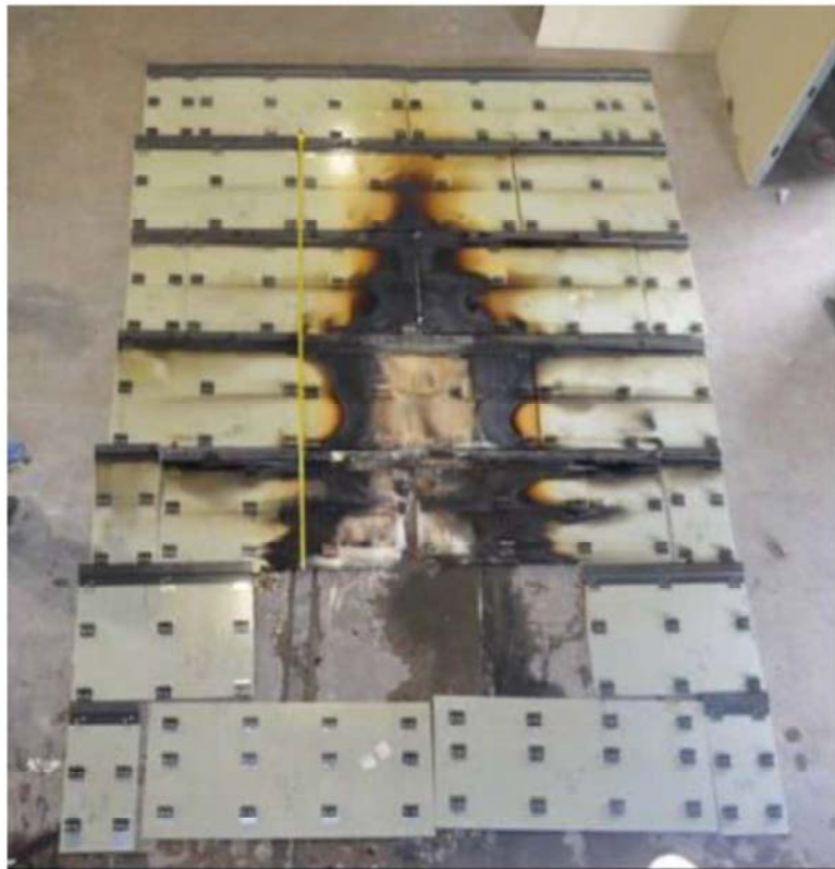
Figure C-17. Post Test Assembly Dissection – Interior Surface of StoneLite® Panels (SP-1-10-3) Panels following Exposure.
